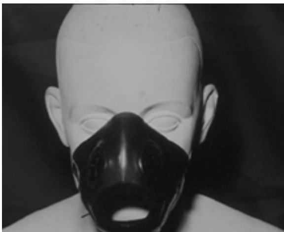
Fig. 16-3. The nosecup of the M45 protective mask has a single, large hole in the center through which exhaled air is expelled on its way to the exit valve in the main mask. Inhaled air, which has passed through the canister, passes up and around the side of the nosecup, preventing fogging of the mask's lenses, after which it passes through the valve (seen on the reader's left) on its way to the soldier's respiratory tract. Photograph: Courtesy of Visual Information Division, US Army Chemical and Biological Defense Command, Aberdeen Proving Ground, Md.
